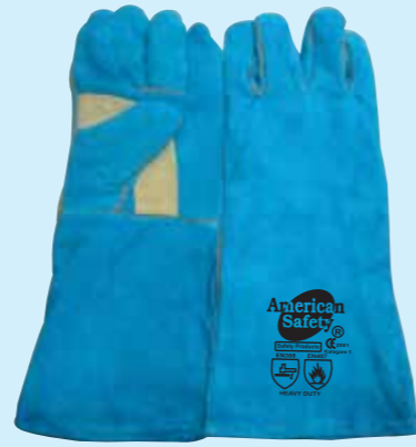
Cow Split Leather Welding Gloves Back Full Pcs. of Leather A Grade Full Inner Flees Lining Full Yellow Leather Piping Covering to Seem Yellow Double Palm for Extra Protection Inside of Cuff Cotton Lining Size : 16" = 40cm CE Approved Comply with EN388 & EN407 Made in Pakistan Art No. : WGGT : 210
