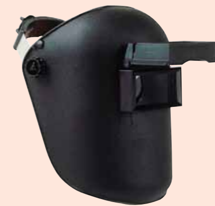
Clip-cap Welding Helmet [ Ce ] [ Ansi Z87 ] (Caps & Lens Not Included) Lift-Front Lens Holder, Lens Size: 4-1/4" x 2" Polypropylene Shell, With ABS Bracket. Art No.: 6PA2
